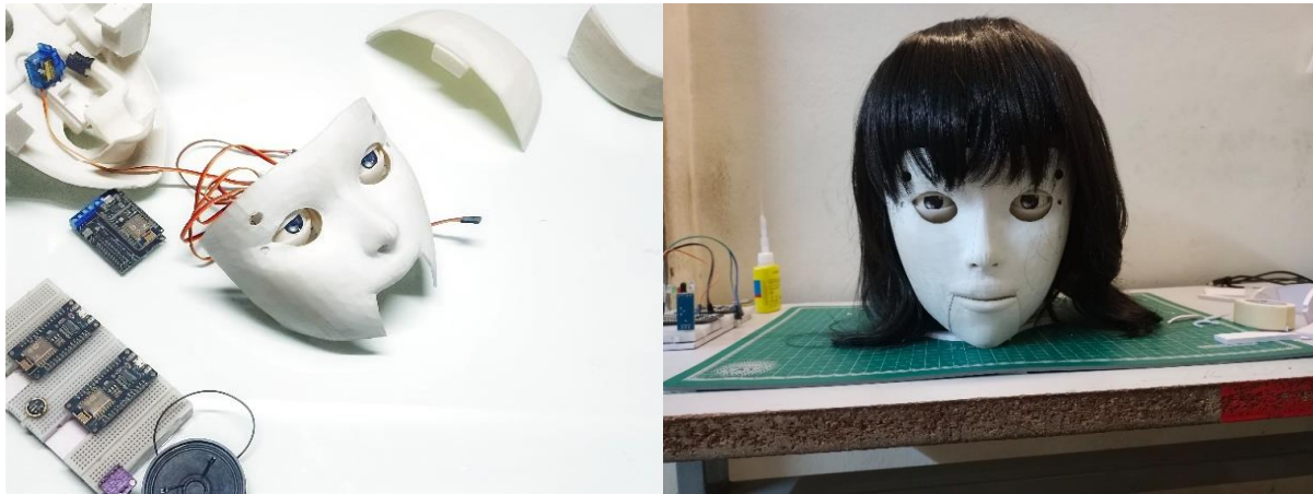
Figure 3: (a) integration of components, (b) final assembly of humanoid robot's head
